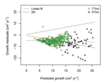
**Figure 7** Growth residuals based on test observations from first-thinning (1Thin) and third-thinning (3Thin) even-sized stands, from simulations with the SD-model (included predictors; S = tree size and D = inter-tree distance), displayed against predicted growth. Trendline from linear regression of both subsets; y = -4.69 - 0.06x (*P*-value = 0.09). Red dotted reference lines display the standard deviation lines from the SD-model calibration (Figure 5).
